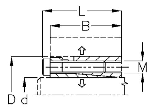
$\begin{array}{lll} \text{B mm} & = 76 \\ \text{d H8 mm} & = 160 \\ \text{D mm} & = 210 \\ \text{Fit tolerance} & = \text{Aksel h8, Nav H8} \\ \text{F kN torque} & = 550 \\ \text{L mm} & = 90 \\ \text{M mm} & = \text{M14} \\ \text{P N/mm2 surface pressure on shaft/hub} = 140 \\ \end{array}$
